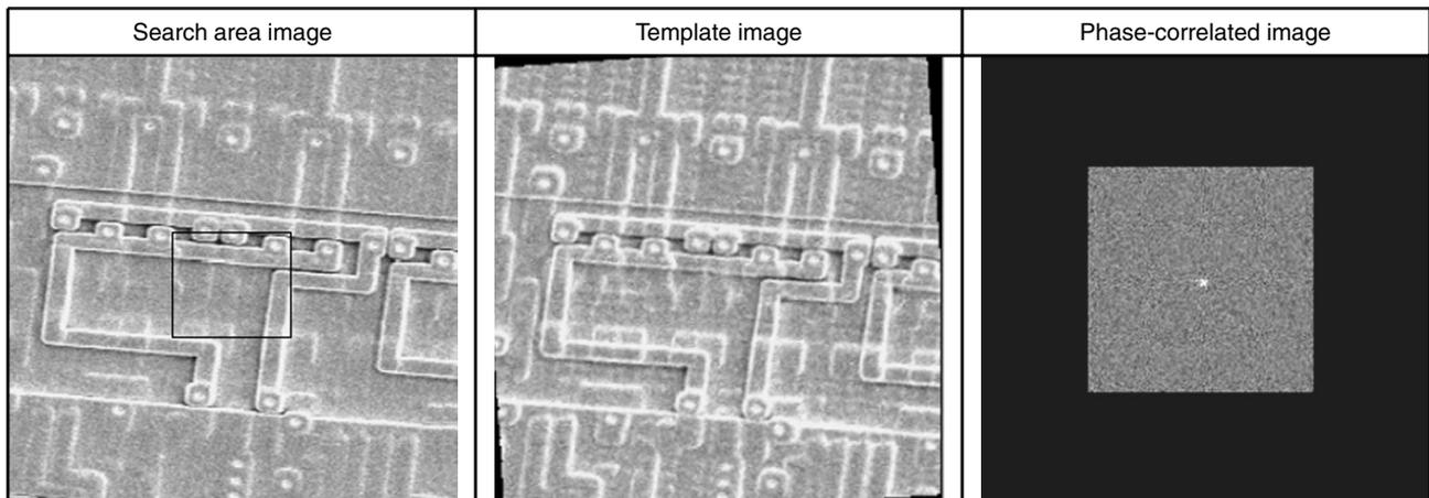
FIG. 5 Images obtained after the die positioning algorithm registers the current scanning electron microscopy image at the failure site of a microprocessor integrated circuit sample. Horizontal field width = 44.6  $\mu\text{m}$ .
