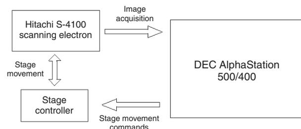
Fig. 1 Block diagram of the automatic die positioning system.
