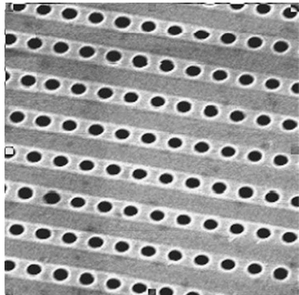
FIG. 3 Scanning electron microscope image of a failure site found on a 16 Mbit DRAM sample. Horizontal field width = 68.3  $\mu\text{m}$ .
